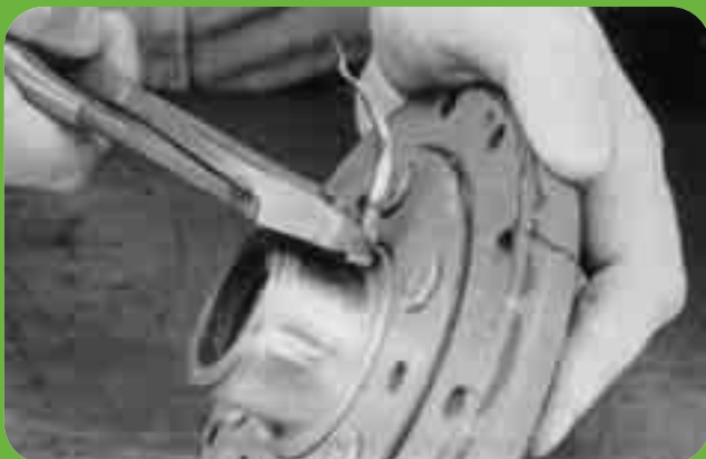
8 Pry flange off installed Speedi-Sleeve®.
