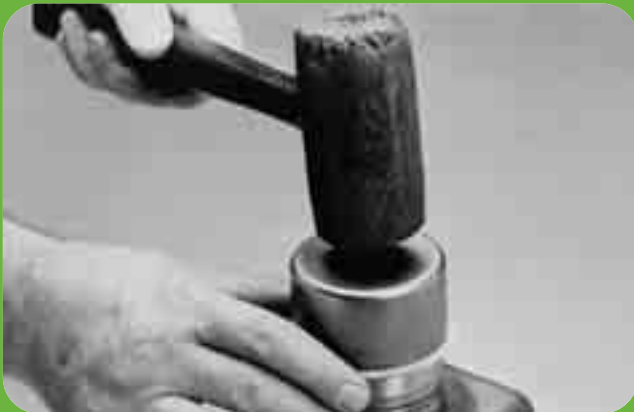
7 Tap tool to install Sleeve over shaft.
