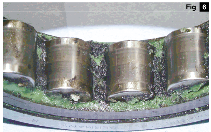
Black discoloured grease affected by current discharges
